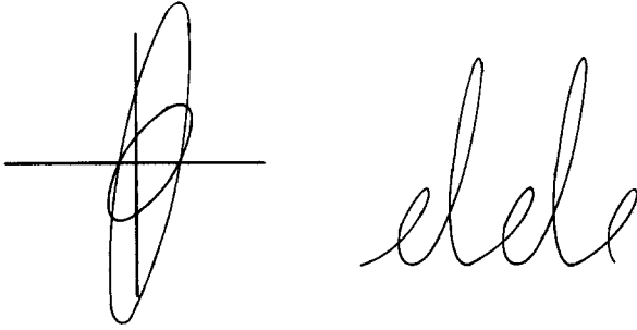
Fig. 4. Modulation of the vertical oscillation at points of zero vertical velocity yields different letter heights by a process of amplitude modulation without phase change
