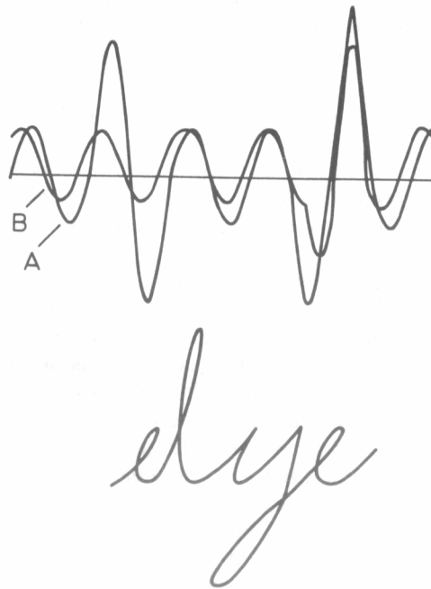
Figure 10.9: Vertical (A) and horizontal (B) velocity components generated by the mass-spring model and the resultant writing trajectory. [From Hollerbach, 1981.]
